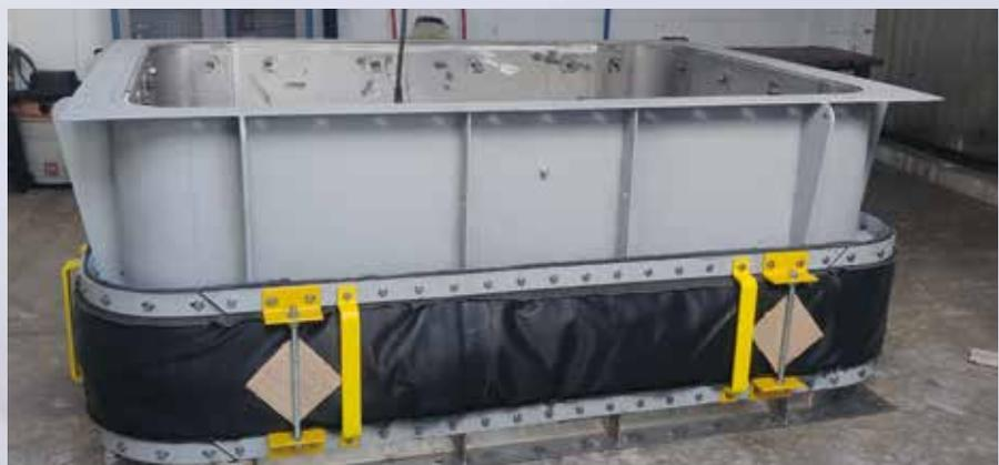
Engineering, manufacturing and installation of the new expansion joint units was completely carried out by EagleBurgmann.
